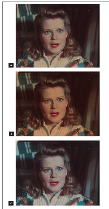
FIGURES 7 (a–c). Comparison of multispectral scans (diffuse illumination) rendered with three different illuminants—(a) high-intensity carbon arc (b) low-intensity carbon arc, and c) xenon light (below)—of an Agfacolor Duplichrome print of the film OPFERGANG (1944). Credit: Gert Koshofer Collection.
