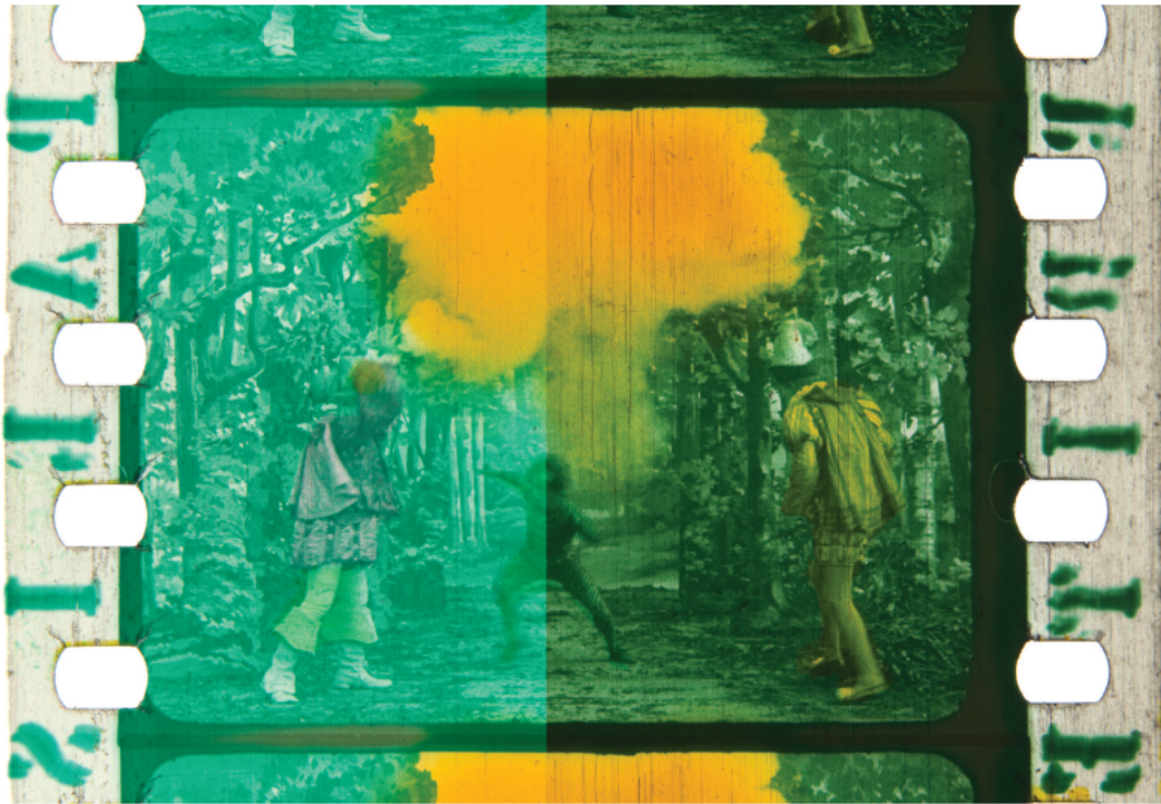
FIGURE 3: Comparison of a stencil-colored and toned film in diffuse (left) and collimated illumination (right) shows the chromatic Callier effect. Multispectral scan of a stencil-colored and toned print of Le Pied De Mouton (1907), Library of Congress, rendered with the spectral emission of a Kinoton FP30 xenon illuminant.
